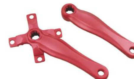
MODEL : LF-1 RED LENGTH: 170MM BCD: 104/64MM
